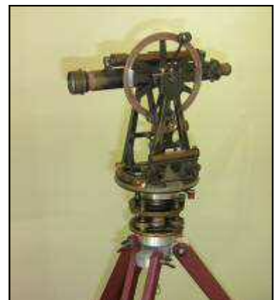
Figure 2 Transit Vernier Theodolite (to be displayed at POP 2013)
