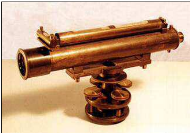
Figure 6 Elementary Dumpy Level made by Baker and dating from the 1850's
