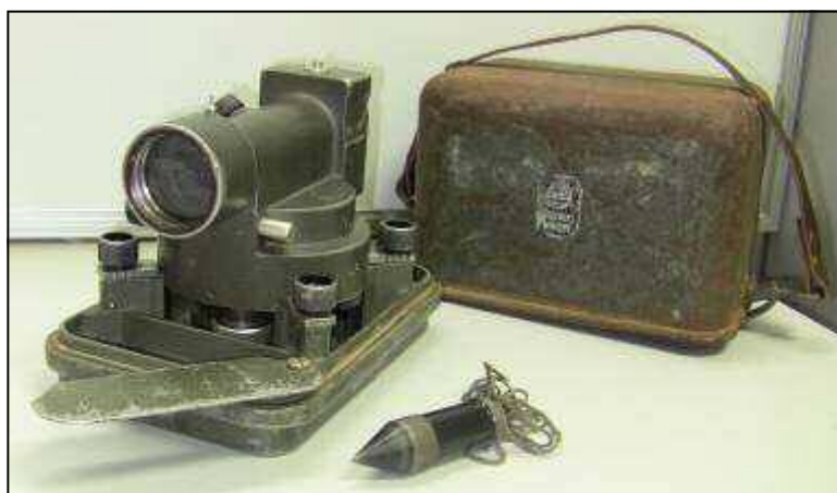
Figure 8 1950's Ertel Compensated Dumpy Level (gift of Bernie Hannan, take a peep through me at POP 2013)
