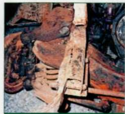
The inner suspension nuts were welded on solidly
