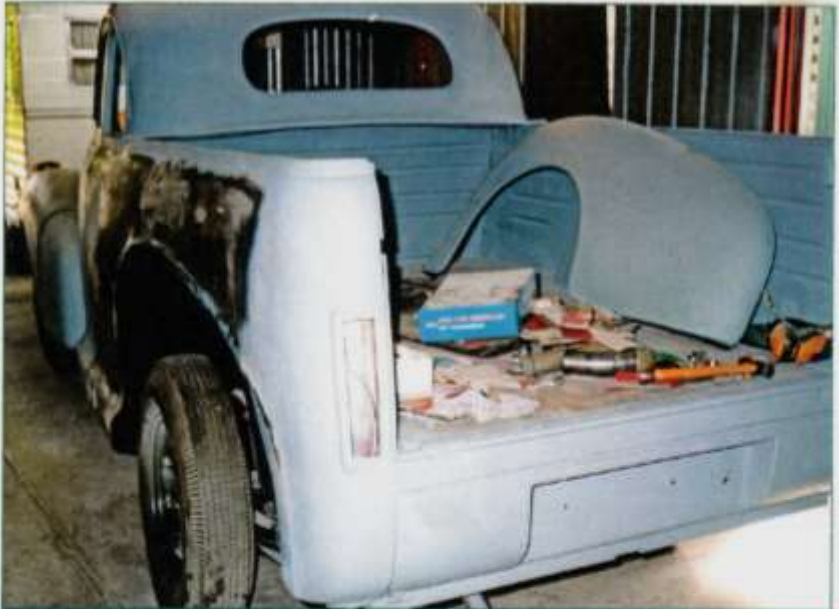
Repairs were made to the body around the wheel arch before the mudguard was attached
