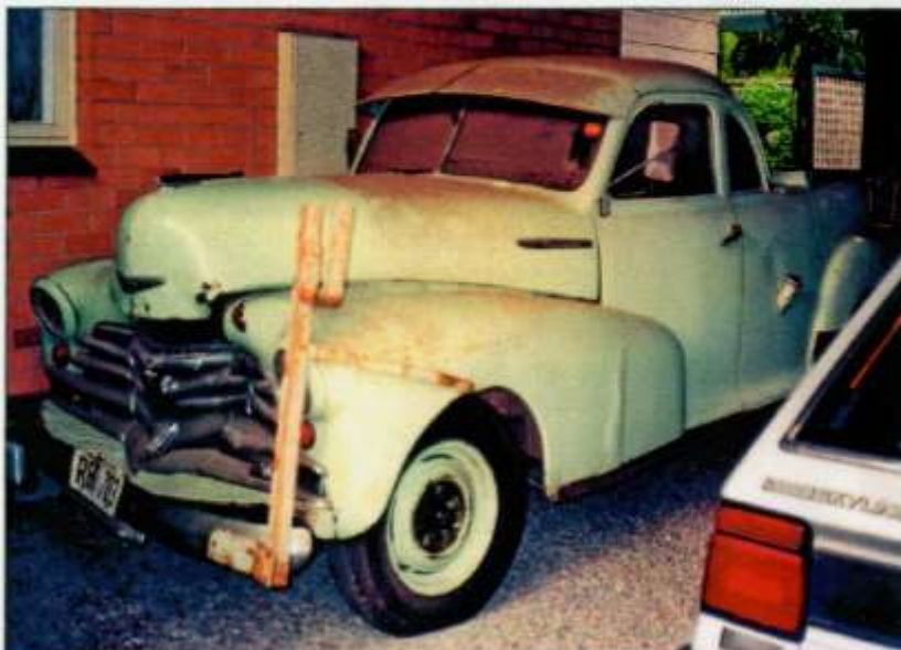
The scaffolding brackets and other 'accessories' were removed first
