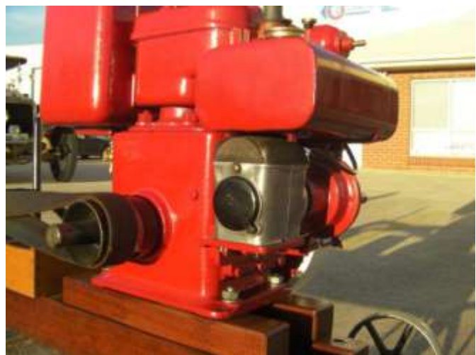
Gane engine showing the vertical mounted magneto
