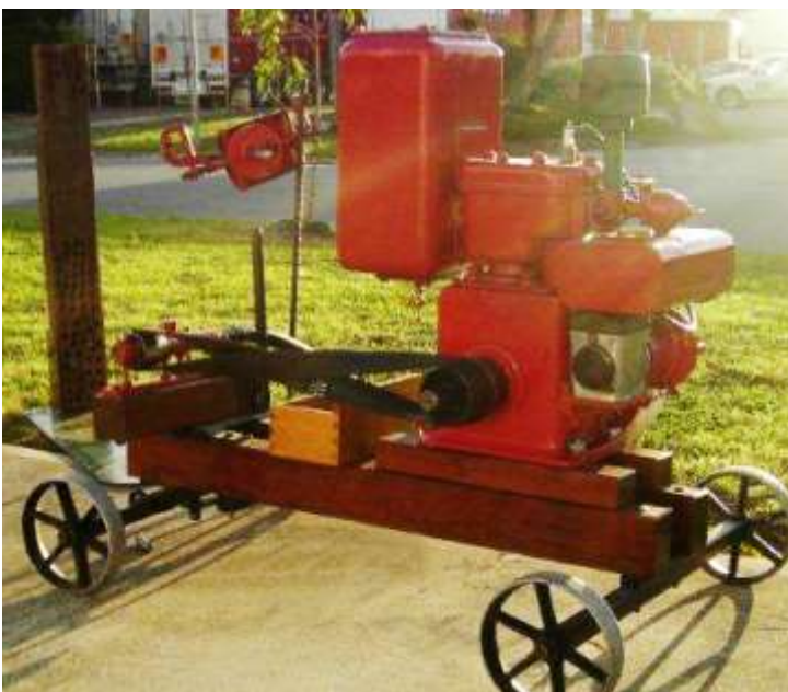
Gane engine with attached Post drill
