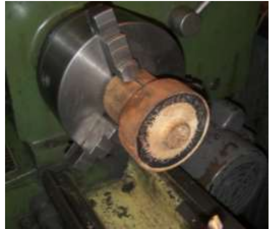
Demonstrates the machined ring sitting in the recessed wooden block in the lathe.
