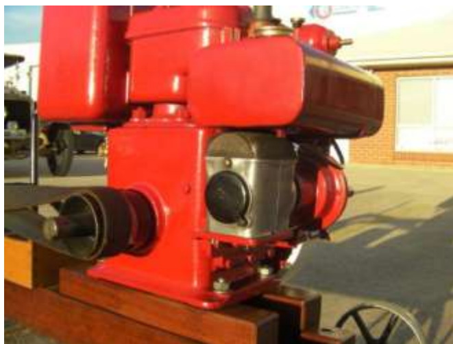
Gane engine showing the vertical mounted magneto
