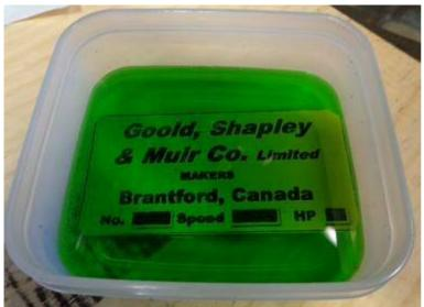
Make sure you are wearing rubber gloves so you do not get an acid burn. After 30 minutes, remove the plate and wash with cold fresh water and dry off with a clean rag. To remove the toner from the non etcher areas, wipe over with acetone a couple of times.
