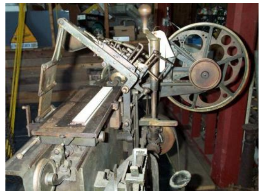
Figure 3 Automated linear dividing engines for making slide rule patterns
