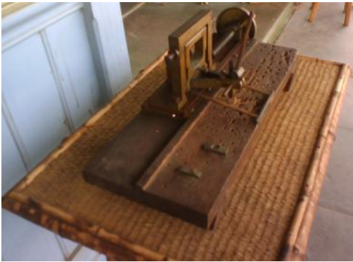
Figure 1 Dividing Engine at Burra antique shop, note vertical scribing tool and holey baseboard for holding down work piece.
