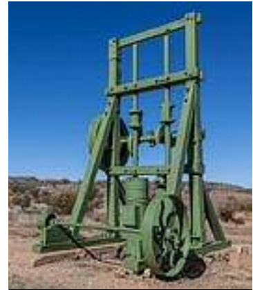
Figure 8 A relict Stamp Battery from USA with "rollers" a bit like Ray's example
