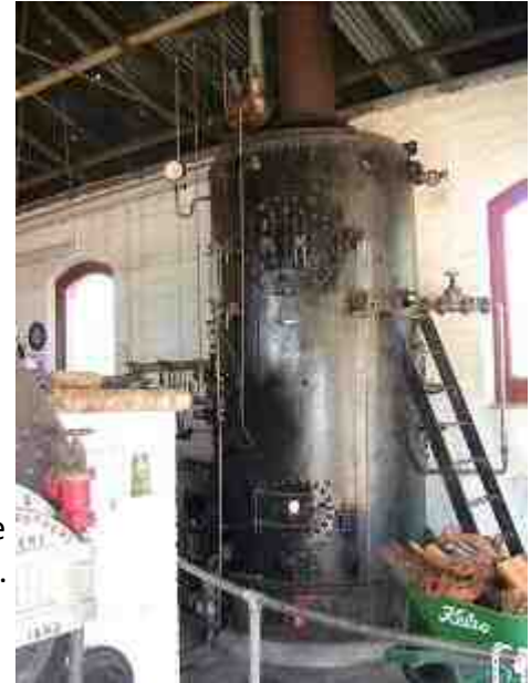
Figure 5 Galloway boiler to provide steam to 1883 Appleby Beam Engine
