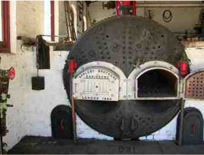
Figure 5 Galloway boiler to provide steam to 1883 Appleby Beam Engine
