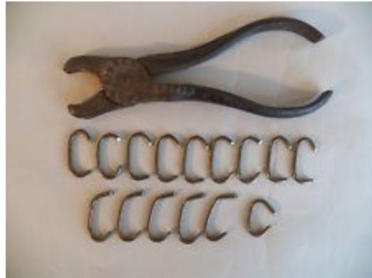
Figure 2 Hog Nose Pliers and clips
