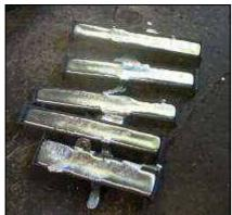
Aluminium pistons or cylinder heads are heated in a large crucible, (a crucible is a pot which is used to hold the molten metal in a furnace) until they reach liquid form. Dross is removed (metal oxides and other scum on the surface of molten metal) and then the molten metal is poured into a mould in the form of an ingot. The ingots are easier to store and use as required.
