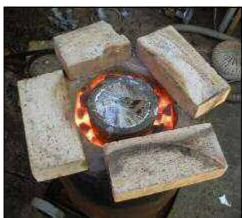
dross is removed again and the crucible is removed from the furnace and placed in a holder tool on a special furnace brick. Then the molten aluminium in the crucible is poured into the sand casting boxes.
