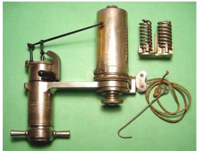
Early brass drum Indicator. Note springs for high and low pressure and lever to exaggerate spring movement.
